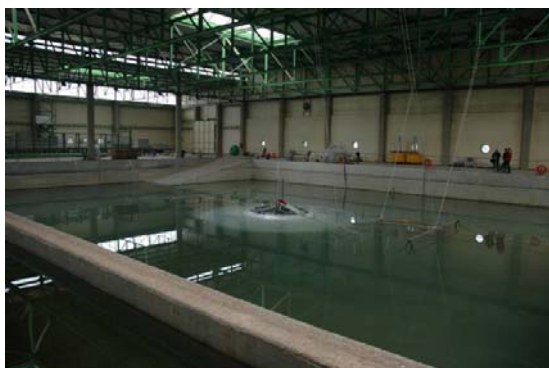
Figure 1. Picture of the conical island placed at the center of the wave tank (left). and a particular of landslide model placed on the ramp (right).
